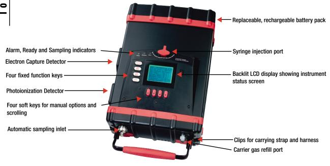
Completely self-contained and convenient to carry, Voyager provides flexibility of analysis, ease of use, and reliable results. Voyager is rugged and water-resistant to handle the toughest environments.
